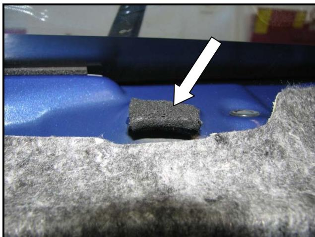
6. After applying the insulating material to each of four (4) tabs, install instrument panel pad assembly in reverse order of removal as per KGIS procedure.
