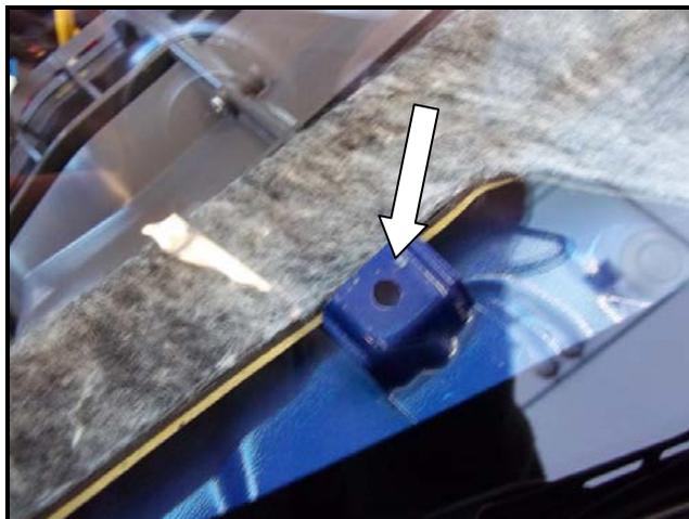
5. Close-up view of insulating material applied to instrument panel pad contact tab.
