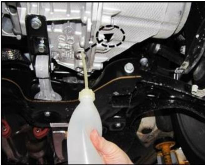
⇐ Insert the tube of the bottle in the marked area (lowest point) of the gearbox housing as shown in the illustration and completely suction out the remaining oil.
