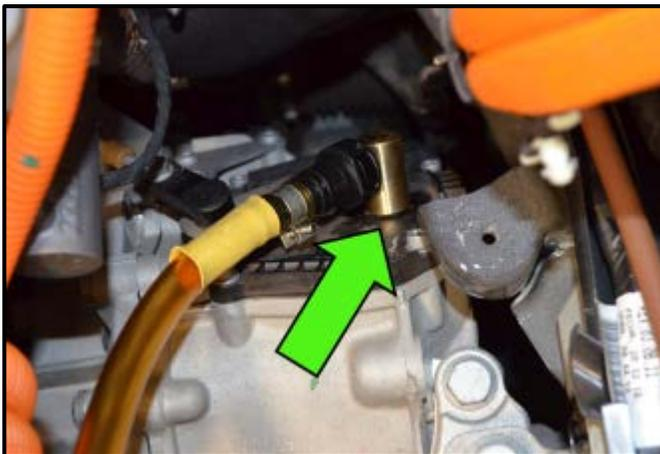
⇐ Install VAS 6262/4 (SET-34F6/1 tool for U.S. dealers) coupled with VAS6262A onto transmission vent as shown <arrow> ensuring that it is fully seated onto the vent to prevent fluid leakage while filling.
