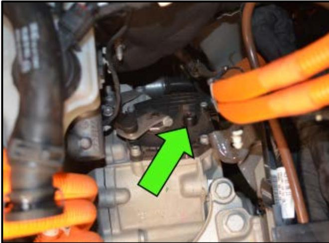
**i** Tip: The location of the transmission vent cap <arrow> is located on top of the transmission near the gearshift lever.
