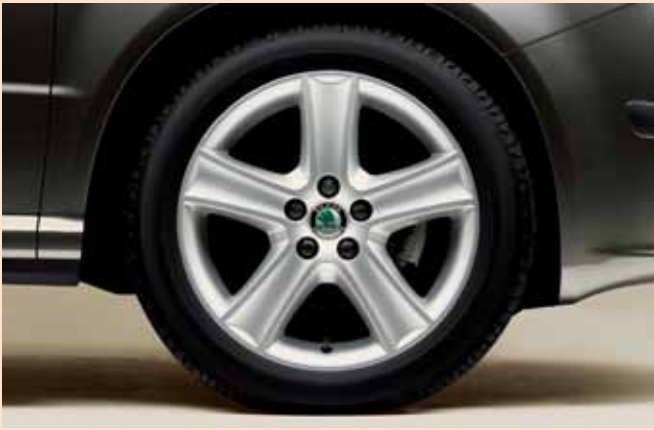
Poli alloy wheels 6.5J x 16" with 205/45 R16 tyres. Extra equipment for the Ambiente and Elegance versions.
