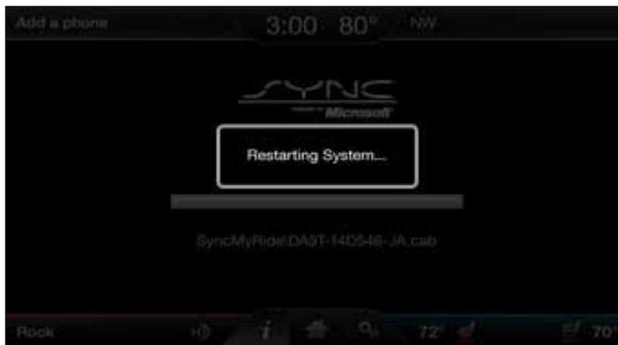
5. At the completion of this part of the process, a “Restarting System” message displays on the touch screen. A reboot will occur during this process.
